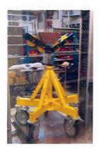
Danish Technological Institute, Certification & Inspection hereby certify that the welding stand with type designation WT FLEXI has been subjected to an overload test with 25% overload = 7500 kg. The product was found to meet the requirements to mechanical stress as stipulated in the Machinery Directive 2006/42/EC (appendix 1, par. 4.1.2.3 b) with revisions and the Executive Order No. 693 issued by the National Working Environment Authority on 10 June 2013 on Design of Technical Equipment.
